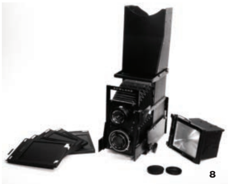
8. Gowlandflex 4x5 "Glamour Camera" Nr. 7020145 with Komura 210mm f6,3 viewing lens Nr. 12065 and Komura 210mm Commercial f6,3 taking lens Nr. 7020145 with Copal Press No. 1 shutter.
